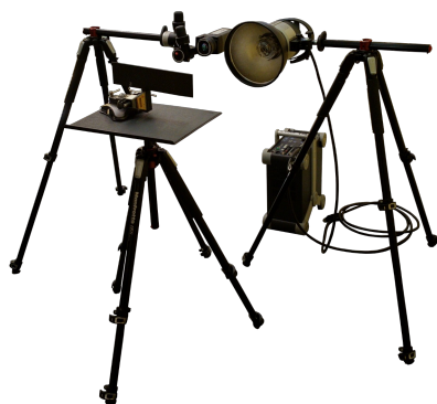
Example of Mounting in Reflection Mode: Overhung pulsed flash heating and camera arrangement enabling closer inspection
