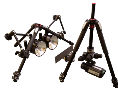
Example of Mounting in Transmission Mode: Sample placed on the floor, with camera and heating positioned upside down.
